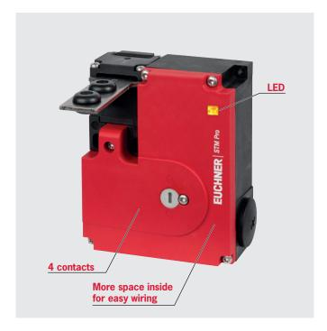
Due to its small design, the electromechanical safety switch STM Pro is suitable, in particular, for applications in which a guard locking function is required in combination with small installation dimensions. The adjustable actuating head with vertical and horizontal actuation opening offers a high degree of flexibility during mounting.
